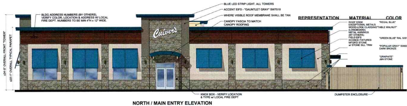
NORTH / MAIN ENTRY ELEVATION
